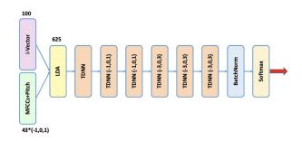
Fig. 8. The architecture of the deep time delay neural network (TDNN)-based acoustic model adopt in the FSR-2020 reference baseline system.
