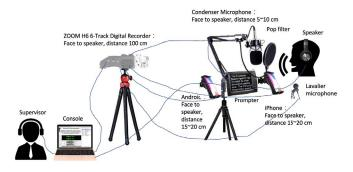
Fig. 3. Schematic diagram of the configuration of the recording equipment.
