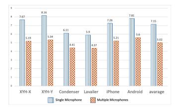
Fig. 9. Performance of advanced TSR system on different microphones on TAT corpus.
